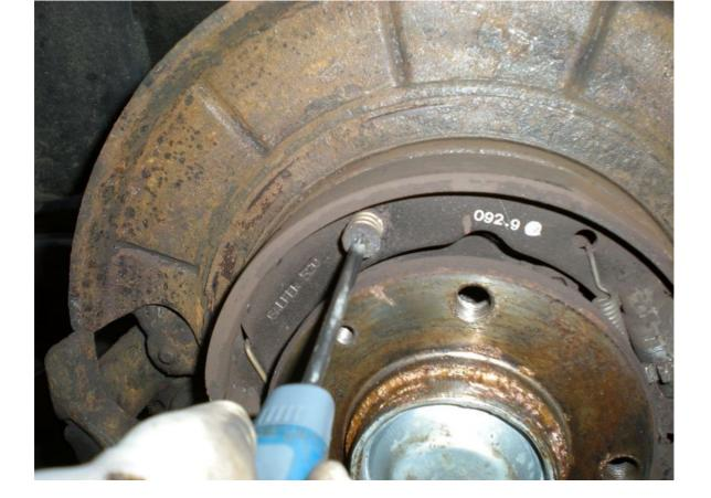
The method I recommend is to use a screwdriver to remove the top end of the spring by the idler first. Don't waste too much time being nice with it, it'll just hurt more. Once the spring is free and safe, pull the shoes apart and take the idler out. Then have a go at the other spring. Watch out because it's under a LOT of tension.
