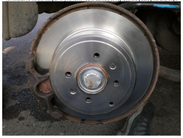
14. Shove your wheel back on. Put a thin film of copper slip on the contact face, so the wheel doesn't seize on. You don't want to be caught at the side of the road with a flat you can't change!
